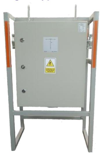
Switchgear type SPR1-AWZ is an electrical device designed for use in the underground mining faces in non-explosive hazard conditions and on the ground in environment 2. Switchgear type SPR1-AWZ is designed for connecting and branching-off mine 3-phase grid circuits with insulated star point on the transformer (IT system) for the grid rated voltage of 500V.
